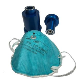
Respirator is now probed and ready for fit testing!
