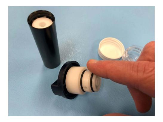
Finally, after the cartridge is fully assembled, blow air on the surface of the alcohol cartridge to remove any dust particles.
