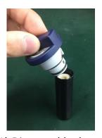
Disassemble the Alcohol cartridge.
