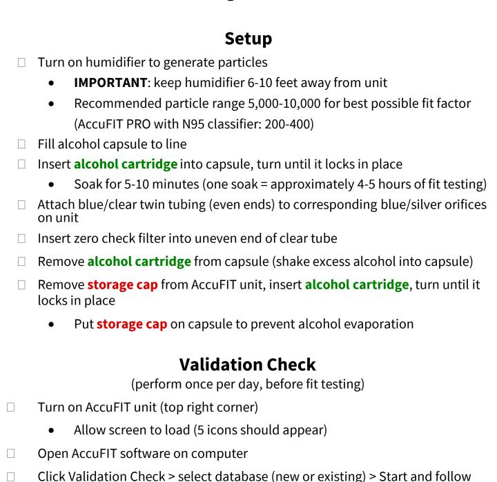
Tip: after connecting the zero check filter, wait 5 seconds before clicking
